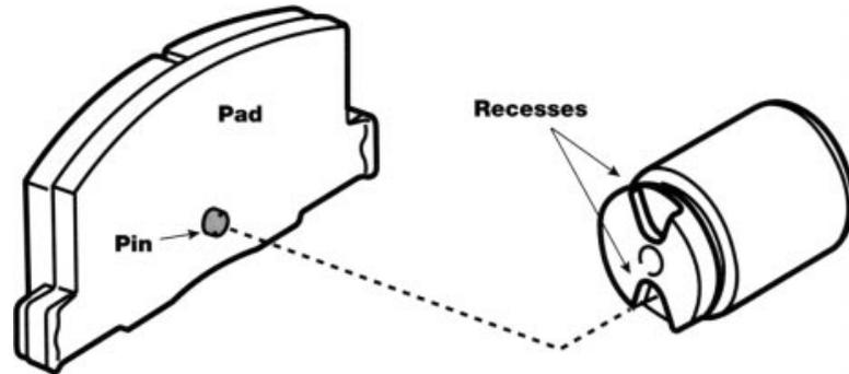
When brake pads are replaced, the piston with the sleeve nut must be forcibly rotated into the cylinder with the Special Service Tool shown below (SST 09719-00020).
