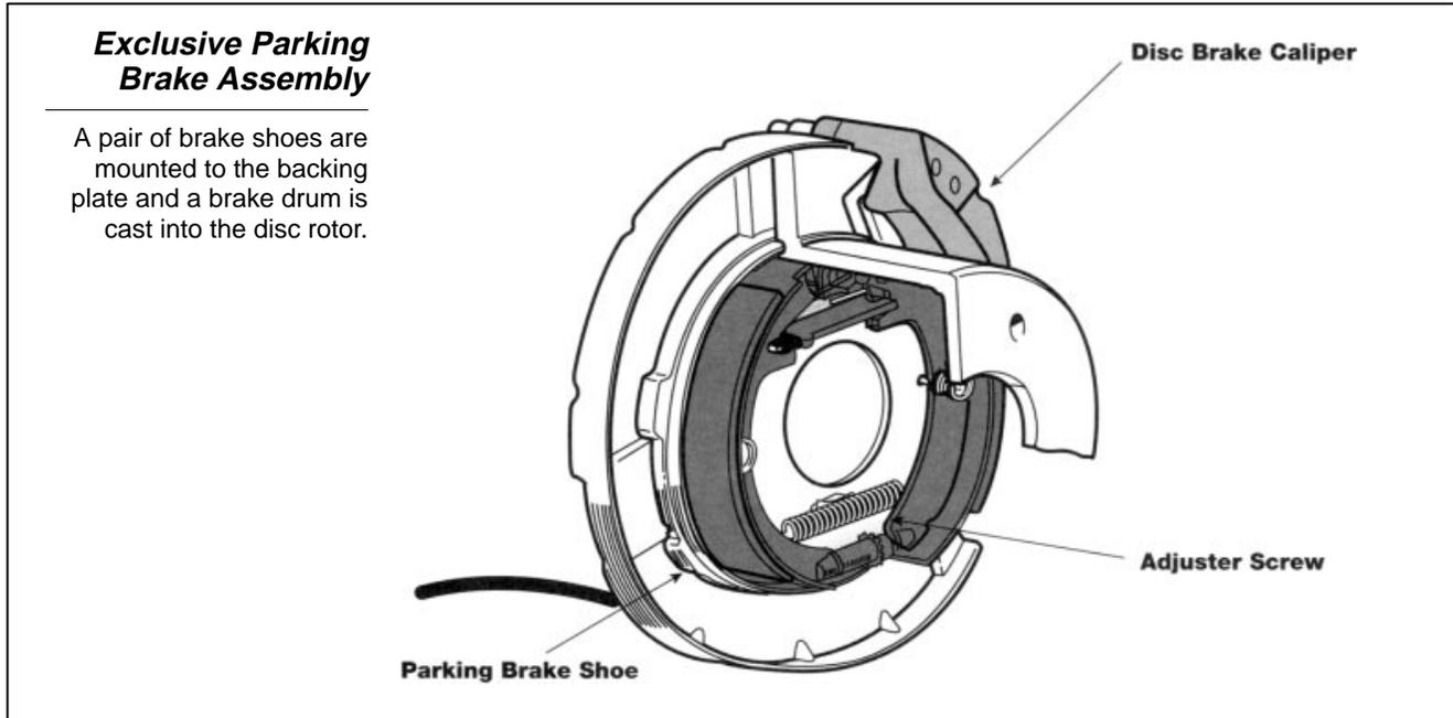
Activating the parking brake is similar to applying the parking brake on conventional drum brakes. Adjustment to the exclusive parking brake is done manually at the Shoe Adjusting Screw Set (Star Wheel) and must be done periodically.
