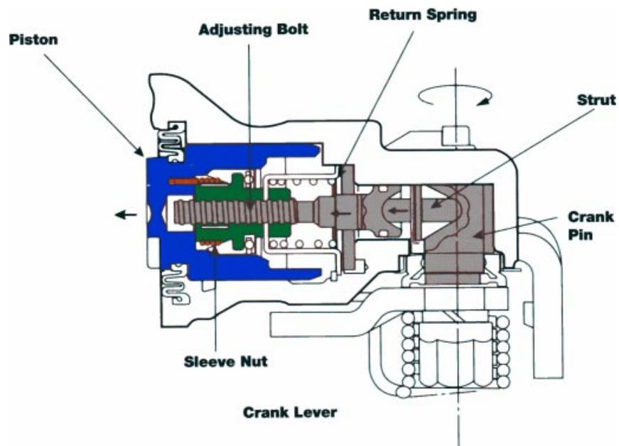
When the parking brake lever is released, the compressed Return Spring pushes the Adjusting Bolt and Piston back to their previous positions. As a result, the parking brake is released.
