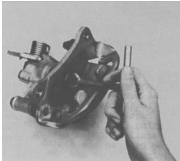
After pad replacement, the parking brake lever travel adjustment should be performed. Depress the brake pedal several times to activate the automatic adjustment within the caliper. Then adjust the cable for the proper number of clicks of the hand brake lever.
