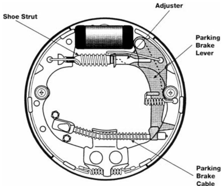
**Disc Parking Brakes** There are two types of rear wheel parking brake systems for disc brakes. The first uses the brake caliper assembly to mechanically apply pressure to the disc. The second type is an exclusive drum brake assembly that applies pressure to an inside drum, which is an integral part of the disc rotor.
